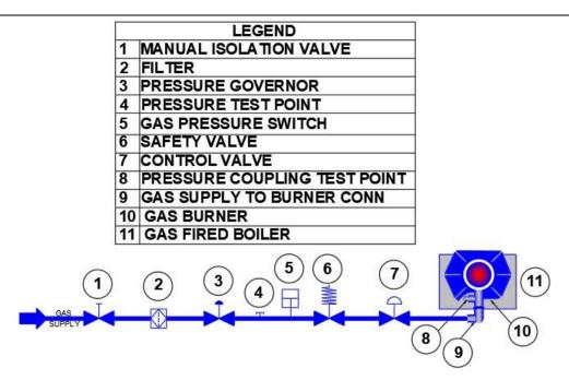
Typical gas supply piping to burner with associated valves and accessories.
