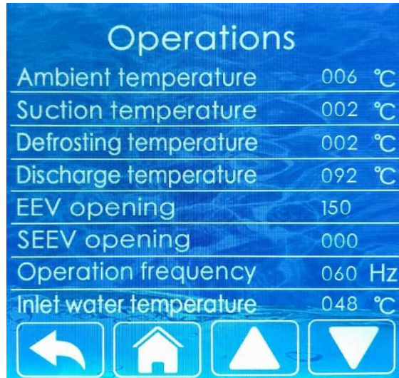
Figure 13 Operation data query interface
